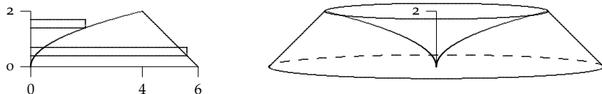
Figure 6.18: Left: The region enclosed by the curves y = \sqrt{x} , y = 6 - x , and the x -axis and two representative rectangles. Right: The resulting solid of revolution about the y -axis (a ‘volcano’) is formed by two distinct pieces each requiring its own integral.
